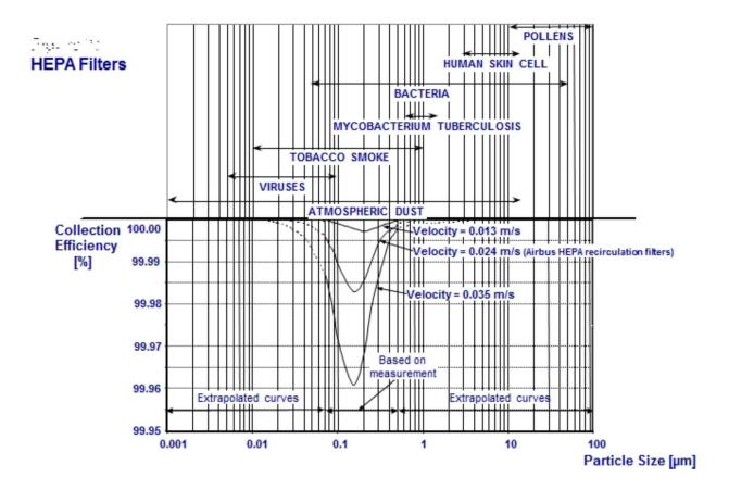
As stated in the attached OIT we consider that the HEPA air recirculation filters capture viruses such as the MERS (Corona virus) and Wuhan Corona virus with extremely high efficiency.
